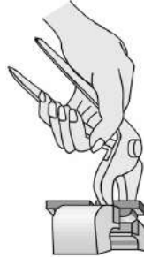
Figure 11. Application of force during radial peeling test.
